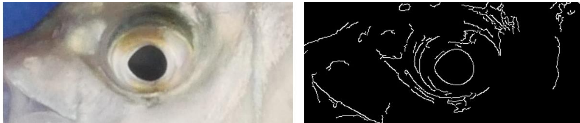
Figure 2a. (Left) Trevally input image: 2b. (Right) Canny edge detection result
